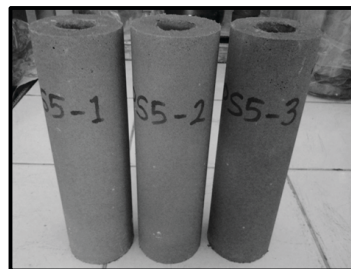
Figure 2. Solid propellant sample
