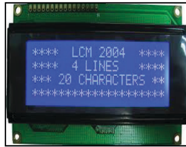
Figure 6. 20x4 LCD display
