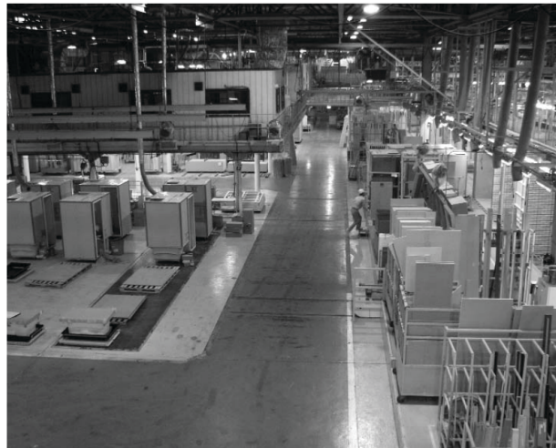
Figure 11 Volumetric module stock in Sekisui House (Source: Hall, Target Magazine, Second Issue 2008, www.ame.org )
