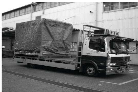
Figure 12 Transporting a volumetric module of Sekisui House (Source: Hall, Target Magazine, Second Issue 2008, www.ame.org )
