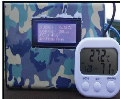
Figure 12. Comparative Test View of SHT11 and Thermo Sensors Digital Hygrometer (Source: Testing)
