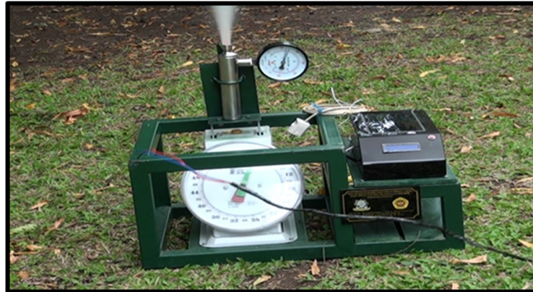
Figure 5. Thrust test tool
