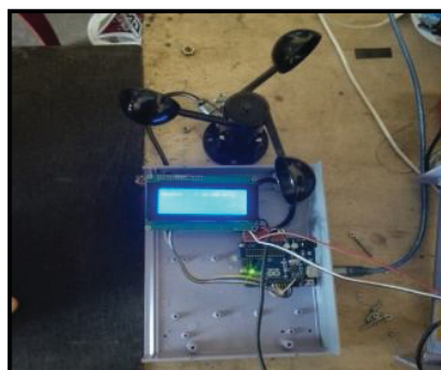
Figure 16. Display Test Sensor Anemometer
