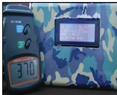
Figure 13. TSL2591 Sensor Comparison Test View and Digital Lux Meter Measure Tool
